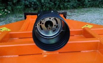
The working width almost equal to the encumbrance, having the transmission to the center of the machine and not sideways, allows to get very close to the obstacles and also to not receive any damage from accidental side impacts of the tool with stones or other.
