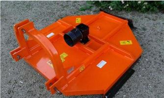
The chain shredder mod. SP is not subjected to the phenomenon of flooding when they proceed with an excessive advancement speed compared to the mass of shredding material. The reason is very simple: the distance between the trenching organs is very large and therefore allows a lot of "dumping", ie the discharge of the shredded material.
