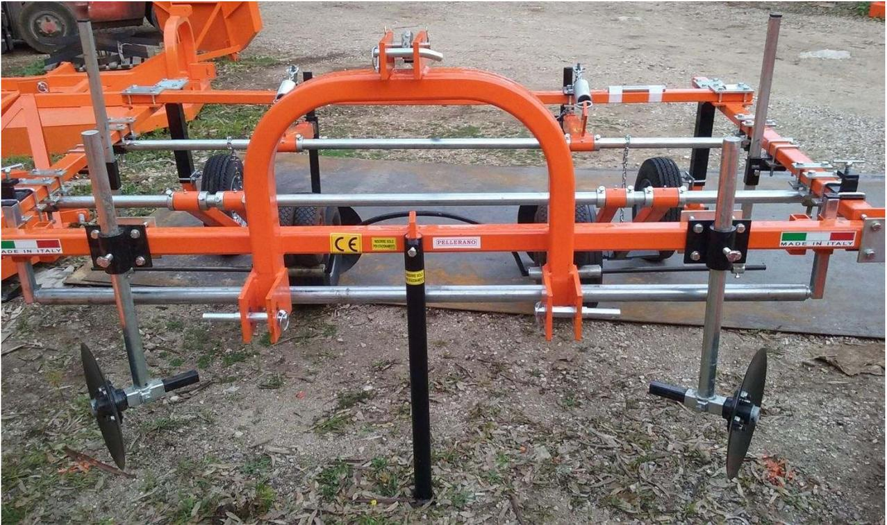
The Stretching Nylon-Mulchers mod.NS extend both the transparent film on the tunnels and the film of mulching.
